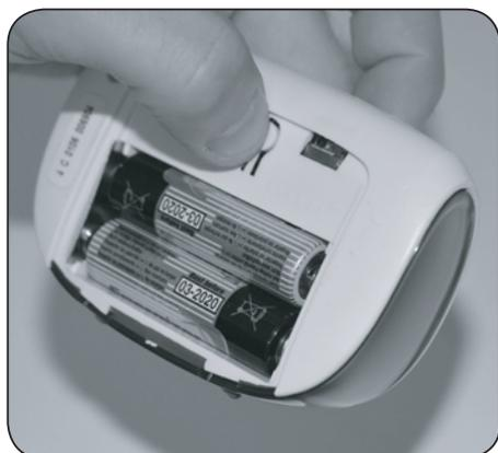
**3.** Still holding the chime replay
