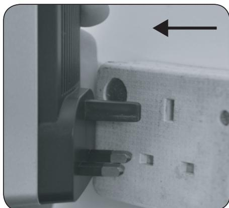
**1.** With the chime unit plugged into a mains socket, either turn off the mains power at the switch, or remove the chime unit from the mains supply.
