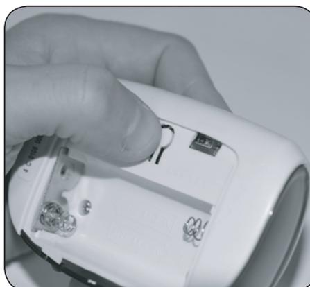
**2.** On the chime unit, press and hold the chime replay
